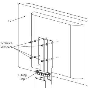
Install your TV onto the bracket, by using a 3mm Hex Allen Key to fasten (4) M4 socket head screws and (4) washers, as shown.
